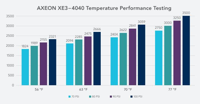
**Note:** To maintain a desired production rate at a lower temperature, increasing the applied pressure may be effective. Ensure that your system and components can safely handle the increased pressure. Consult with a technician to confirm that adjustments are within safe operating limits.
