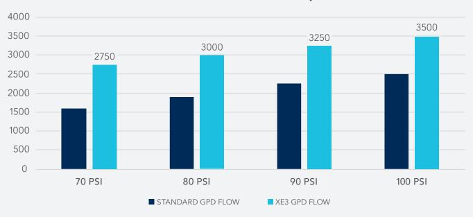
**Warranty Evaluation Test Conditions:** Permeate flow and salt rejection based on the following test conditions: 550 ppm, filtered and dechlorinated municipal tap water, 77 °F / 25 °C, 15% recovery 4040 at the specified operating pressure. Minimum salt rejection is 96.0%. Permeate flows for warranty evaluation may vary +/-20%.
