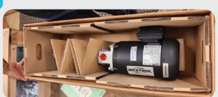
Place extra support all around the pump to keep it in place. There should be very little, if any, room around the pump when these supports are in place. These can be pieces of cardboard or flat foam packing materials.
