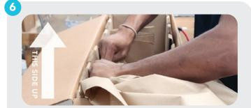
Add kraft paper or some other sort of packing material over the entire unit. Pack as tightly as possible to avoid any movement in transit. Do not use packaging peanuts.
