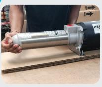
Please make sure that there is no residual water left in the pump because this can create damage to the box during transit. Cap off the inlet and outlet ports to prevent any water from spilling out. Bolt the pump down to a sturdy cardboard or wood base depending on the size of the pump. If the pump has a capacitor, be careful when positioning to leave just enough room on the side of the pump to fit it in the box.
