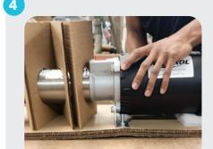
Add protection to the pump end. Premade cardboard pieces are optimal, but any material should be sufficient as long as the pump has cushioning all around it. Depending on the length of the pump, you may need more material.
