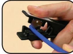
Cut the tube square and remove burrs and sharp edges. Ensure that the outside diameter is free from score marks. For soft or thin-walled plastic tubing we recommend the use of a tube insert.
