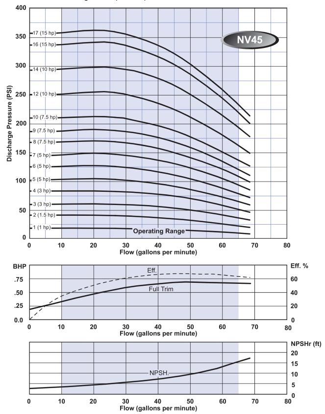
Curves are based on 60 Hz 3450 rpm motors. 50 Hz 2875 rpm curves are available. These curves are for general guidance only, individual pump curves are available upon request. A certified curve may be requested for an additional cost. Webtrol will build pumps to fit your specific needs, contact factory for pricing.
