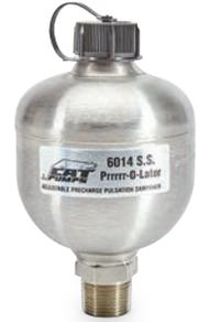
A pulsation dampener contains a dry nitrogen charged bladder that is used to absorb both the high and low fluctuations of pressure produced by a positive displacement pump. A pulsation dampener's bladder not only absorbs the pressure spikes during operation, but due to the nitrogen charged bladder, it pushes flow back into the stream during the low pressure wave, reducing the total fluctuation to 2–3% when properly sized.
