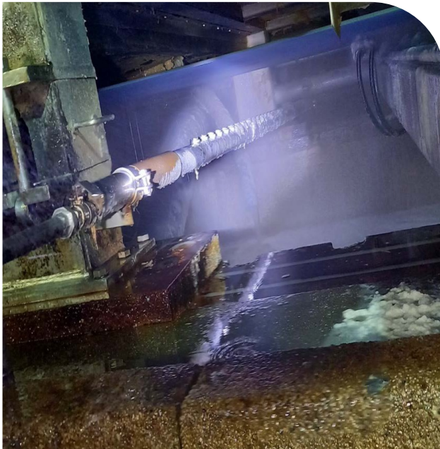
Spray bar beneath forming wire
